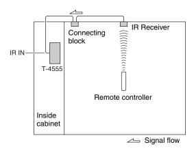
Connect the IR receiver to the T-4555 as shown below.
